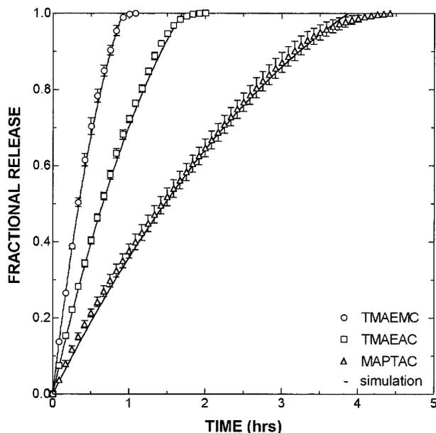
**Figure 4** Effect of type of quaternary amine groups on the release of sulfathiazole from tablets of drug-polymer complexes consisting of 50 mol % MMA at pH 7 (0.2M NaCl).
