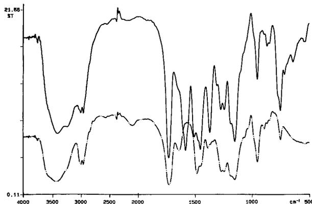
**Figure 1** FTIR spectra of drug-free PTMAEMC/MMA (— · — ·) and diclofenac-PTMAEM/MMA complex (—).
