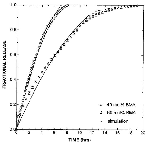
**Figure 3** Effect of copolymer composition on the release of sulfathiazole from tablets of drug-polymer complexes consisting of PTMAEM/BMA at pH 7 (0.2M NaCl).
