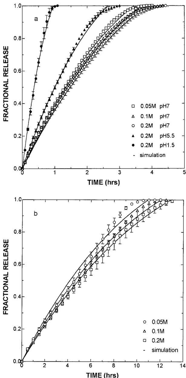
**Figure 6** Effect of pH and ionic strength on the release of drugs from tablets of drug-polymer complexes consisting of PMAPTAC/MMA (50/50): (a) sulfathiazole and (b) diclofenac.
