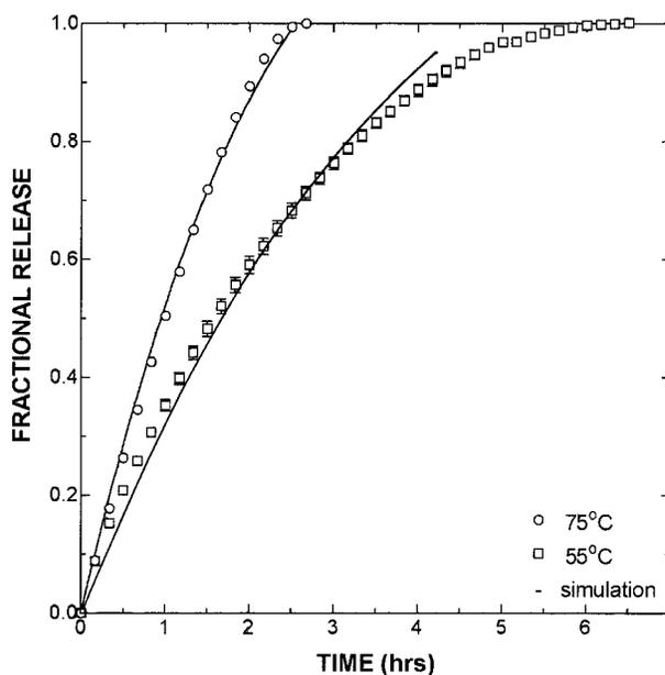
**Figure 5** Effect of polymerization temperature on the release of sulfathiazole from tablets of drug-polymer complexes consisting of PTMAEM/MMA (40/60).
