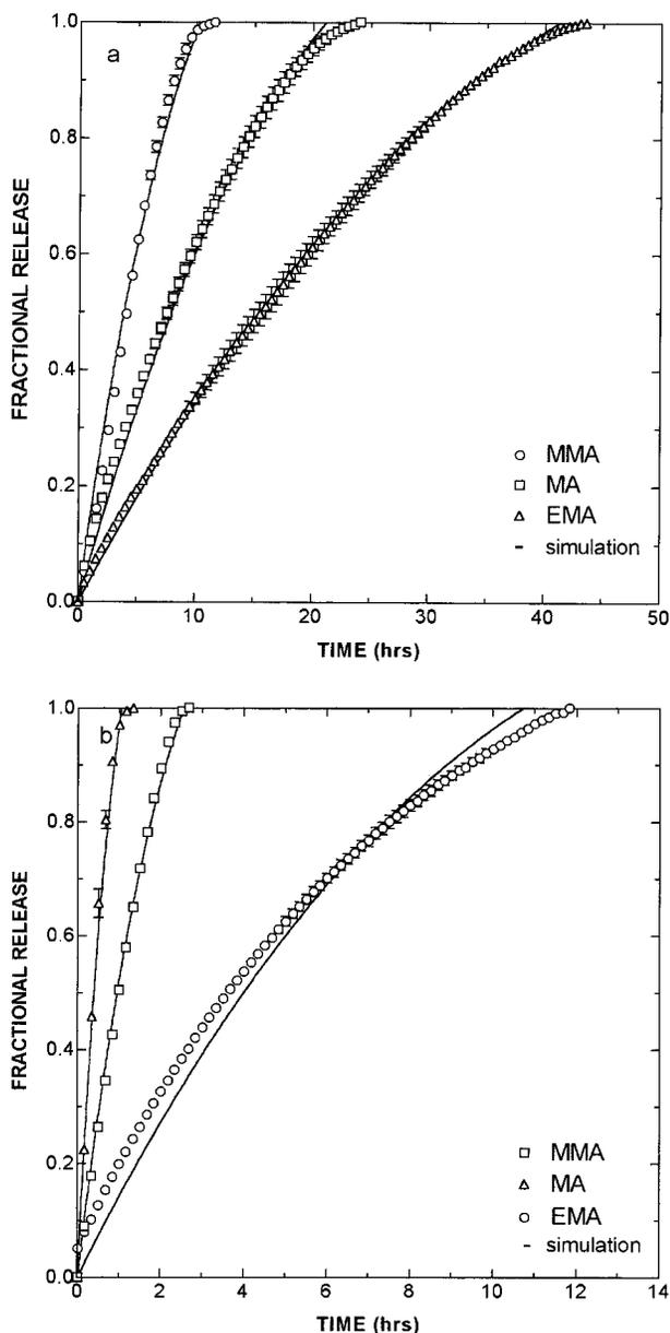
**Figure 2** Effect of hydrophobic groups on the release of drugs from tablets of drug-polymer complexes consisting of 40 mol % TMAEMC at pH 7 (0.2M NaCl): (a) diclofenac and (b) sulfathiazole.
